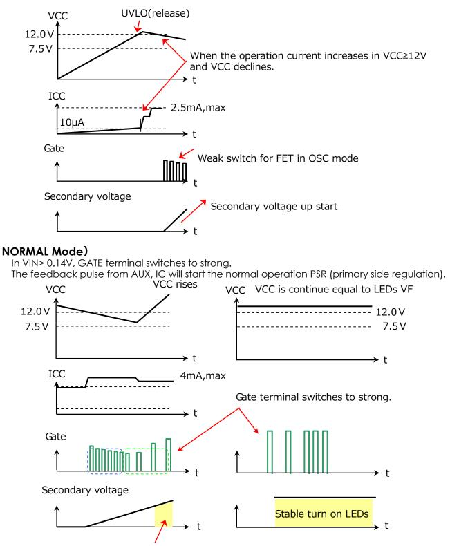
When the secondary voltage over LED's VF, LED start to turn it on.
