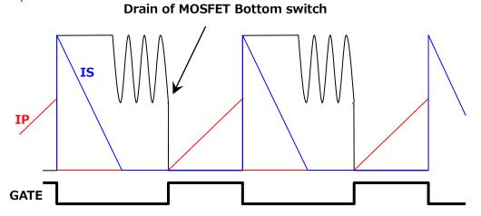
This resonance-amplitude is related to the VF of the LED and primary secondary turn-ratio Ntr. Drain resonance amplitude(V) = VF \* Ntr
