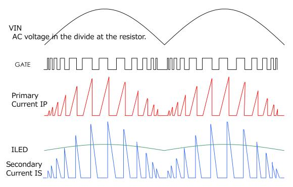
Because the main system is single stage PFC, the LED current waveform of the secondary side includes a ripple. To make LED current waveform smoother, it makes a secondary output capacitor big. The GATE pin is modulating a frequency.
